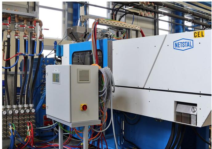
The switch cabinet also contains Eaton's XI/ON modular I/O system which handles the data exchange with the locking system of the guard door, the position sensors or between the tool and the injection molding machine.
