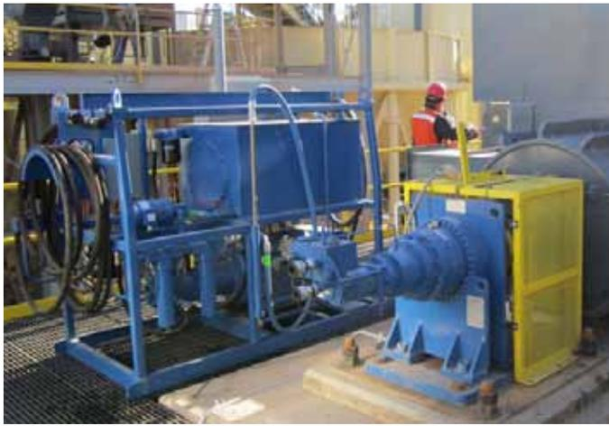
*Eaton's new hydraulic inching drive includes a 75-horsepower hydraulic power unit skid and an Eaton Char-Lynn 6000 Series hydraulic drive motor.*
