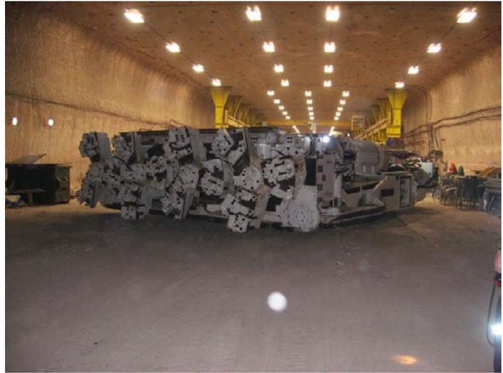
An Eaton Hydrokraft motor is the heart of the hydraulic system on PCS's new X CEL miner that extracts some 1,200 tons of potash per 100 feet of advance per hour.
