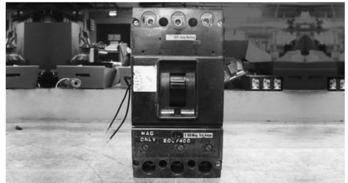
**Figure 14. HKAM Mining Breaker Modified by Third-Party Refurbisher**
