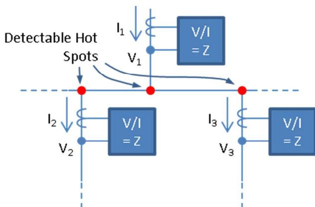
Fig. 10: Measurements of  $V$ ,  $I$  and  $\phi$  at each of these three meters provides sufficient data to detect hot spots on the bus interconnecting these meters.
