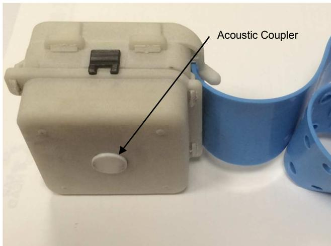
Fig. 8: Piezoelectric Acoustic Sensor with mounting strap and acoustic coupler.
