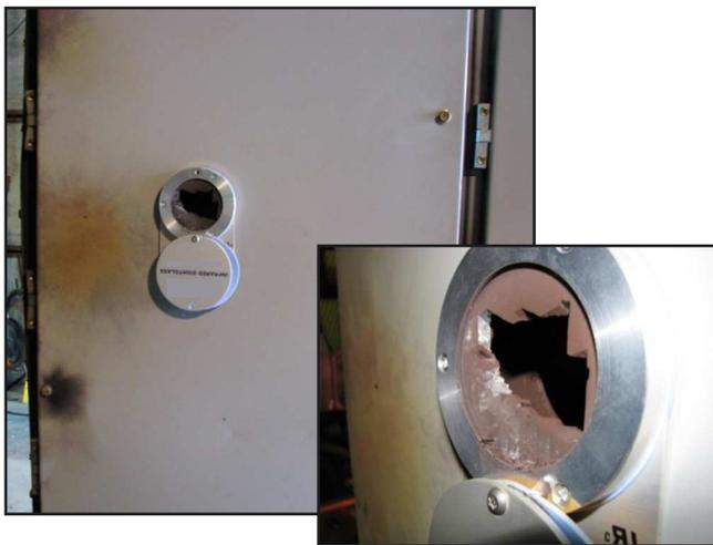
Fig. 5: IR window failure occurring during an arc test of a MV motor control center incoming line compartment.
