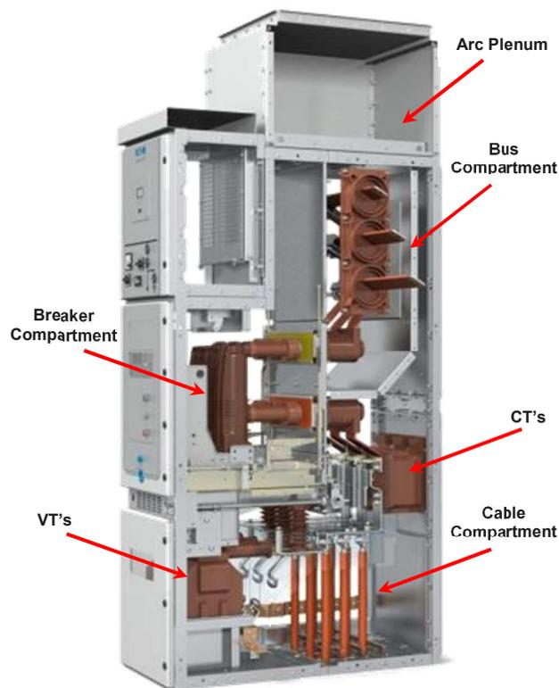
Fig. 4: Typical internal arc classified MV IEC switchgear assembly. Each section is compartmentalized leaving few locations where IR windows could be effectively applied.
