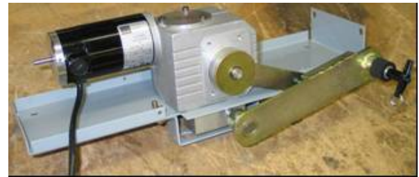
Figure 13. New remote switching on MV Motor Starter Isolation switch
