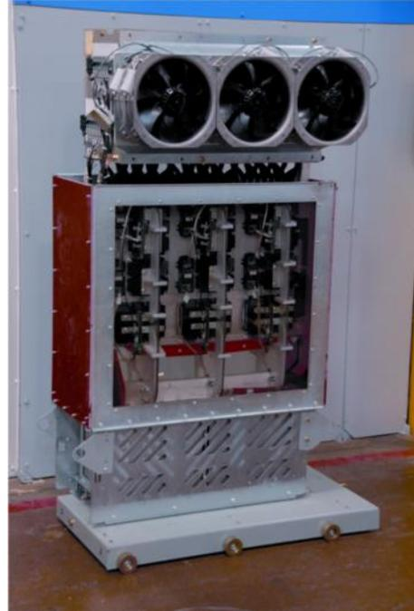
Fig. 6: VFD Inverter Subassembly
