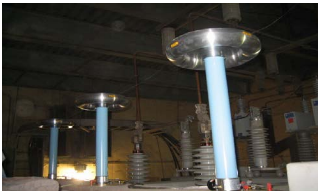
Figure 3. (a) The voltage dividers installed at LMF1 primary, (b) The transient recorder and grounding for LMF1
