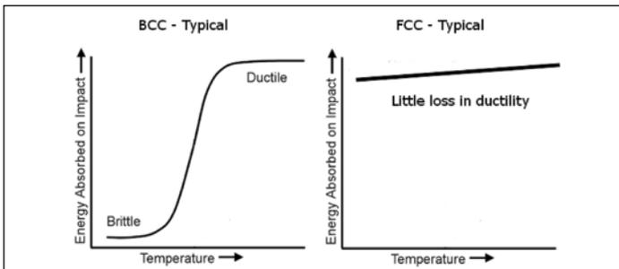
**Figure 3. Ductile-Brittle Transition**
