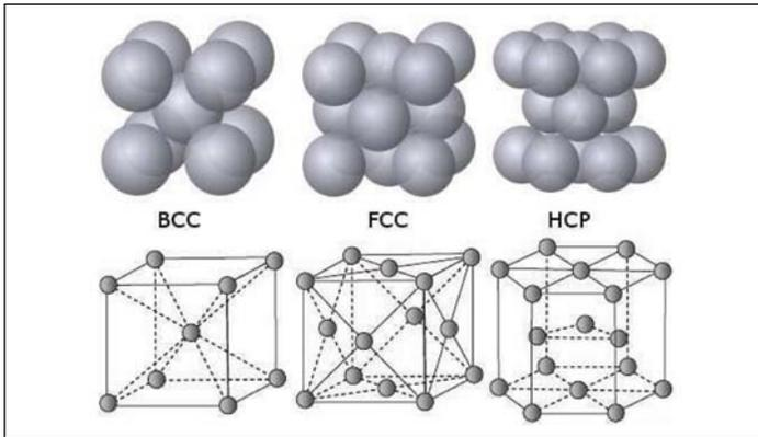
**Figure 2. BCC, FCC, HCP Crystal Lattice Structures**
