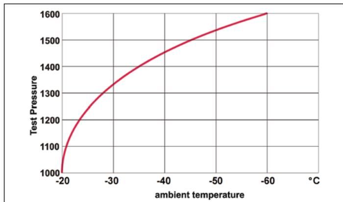
**Figure 1. Increase of Test Pressure (kPa) for Ex d Enclosures at Low Ambient Temperatures**
