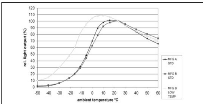
**Figure 4. Relative Light Output vs. Ambient in Hazardous Location Fluorescent Luminaire with Different Lamps**
