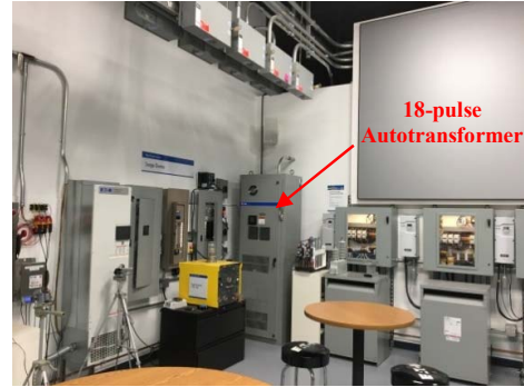
Figure 16: Experimental “windmill” 18-pulse ASD system setup.
