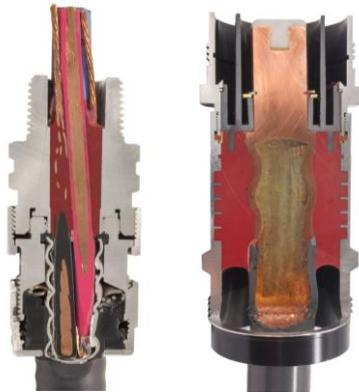
Fig. 15 Liquid seals for a cable gland and a cable connector showing good fill and robust seal.
