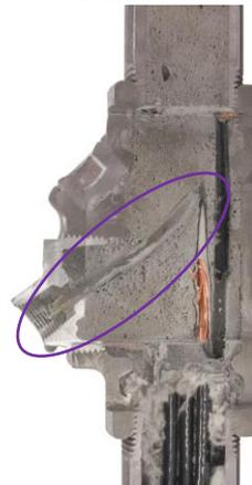
Fig. 12 Drain seal fitting showing the lack of any draining capability when the drain tube is covered with sealing compound.
