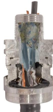
Fig. 16 An example of a poorly installed putty seal. Notice the mottled appearance from incomplete mixing of the putty and the gaps in the seal where flames, gases and vapors can potentially pass.
