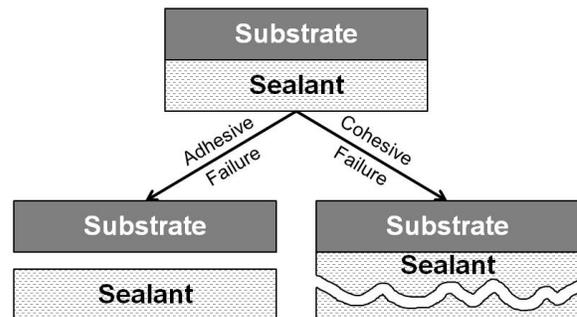
Fig. 10 Diagram showing both adhesive (left) and cohesive failures (right).
