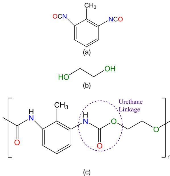
Fig. 8 Polyurethanes (c) are prepared from a diisocyanate - NCO (a) and a polyol -OH (b).
