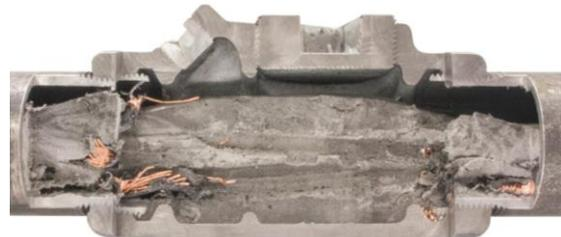
Fig. 11 Foaming polyurethane seal poured below the recommended temperature. The low temperatures limited the foaming reaction resulting in an insufficient seal near the top of the fitting.
