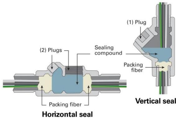
Fig. 4 Horizontal (left) and Vertical (right) seals showing the placement of the packing fiber.
