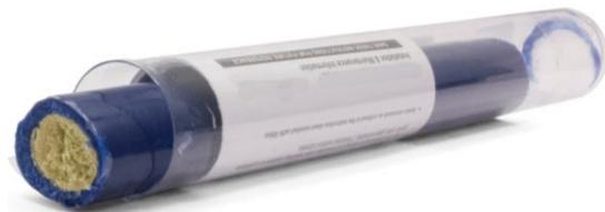
Fig. 6 Putty type epoxy sealant, the “rope” contains both parts of the epoxy. Simply cut the desired amount, knead according manufacturer’s recommendations and install.
