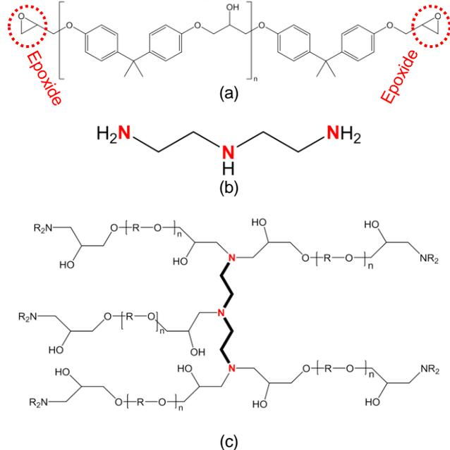
Fig. 5 Examples of reagents for an epoxy resin (a), hardener resin (b), and a cross-linked epoxy (c).
