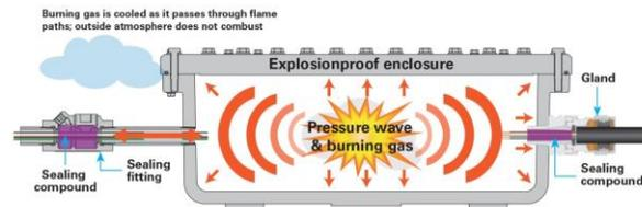
Fig. 2 Diagram showing the operation of an explosion-proof enclosure and the function of conduit cable gland seals, though a cable connector performs the same function of limiting the passage of gases and vapors and prevent the passage of flames.
