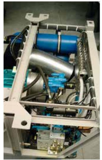
Eaton’s Hydraulics Power Units contain PVM piston pumps, slip-in cartridge valves, servo valves and Eaton’s filtration products HP.170 and HP.91
