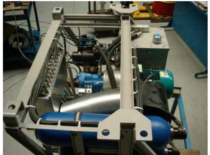
Eaton's powerful Hydraulic Power Unit containing PVM piston pumps, slip-in cartridge valves, servo valves and Eaton's filtration products.
