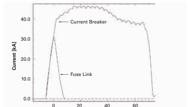
Record of proving tests, showing HSCB and fuse link on same graph.
