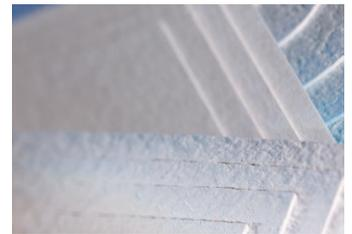
**BECO KD 7** depth filter sheets consist of finely fibrillated cellulose fibers from deciduous and coniferous trees that provide an especially high water-retention capacity.
