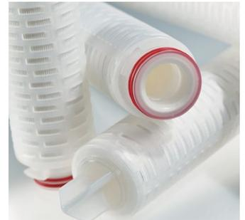
**BECO MEMBRAN PS Pure™** membrane filter cartridges safely retain spore-forming bacteria, which can harm fruit juice, using an asymmetric pore structure with an LRV (log reduction value) of more than 7 per cm<sup>2</sup>.
