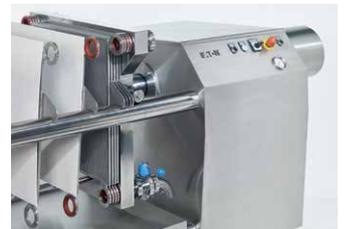
The **BECO COMPACT PLATE A600 sheet filtration system** is a high-quality, multi-layer filter with a variety of options. The filter surface can be adapted to the respective application, and drip loss reduced to a minimum through the hydraulic tightening unit with automatic subsequent pressing.
