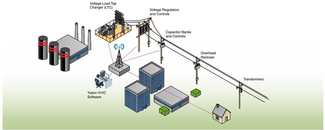
**Figure 1.** Typical diagram illustrating how Yukon IVVC application works within a power distribution system.
