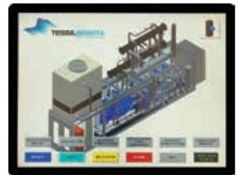
The Micro Panel XV400 provides an overview of the plant and its local and remote components.
