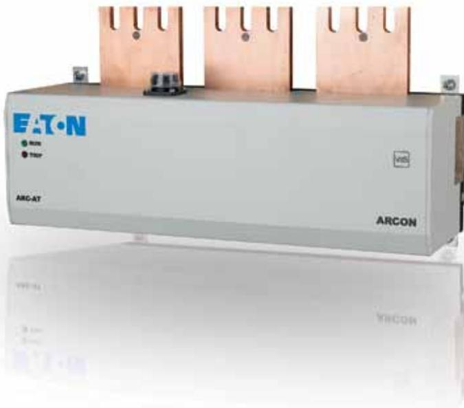
If both the sensor and logic module simultaneously detect a current exceeding defined thresholds, an extinguishing device is triggered. This device initiates a three-phase short circuit as close as possible to the feed point, in parallel with the fault location. The current takes the path of least resistance and the arc fault is extinguished. Thus, the energy that would otherwise have fed the arc is diverted to the short circuit, stopping the arc before it has a chance to develop.
