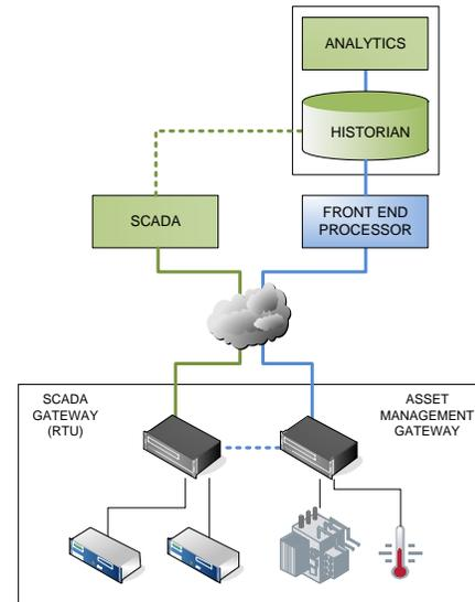
Figure 2: Parallel data path for non-operational data
