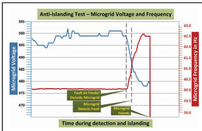
Figure 1 demonstrates microgrid controls developed for anti-islanding capability. Frequency and voltage deviation generated by the controller allows the protection relay to open the microgrid interconnection switch. This allows the microgrid to isolate from a faulted line and power loads within the microgrid while safely allowing service personnel to work on the faulted line.
