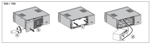
Warning: take care not to inverse the polarity + (red) and - (black) when connecting the batteries as this will destroy the device.
