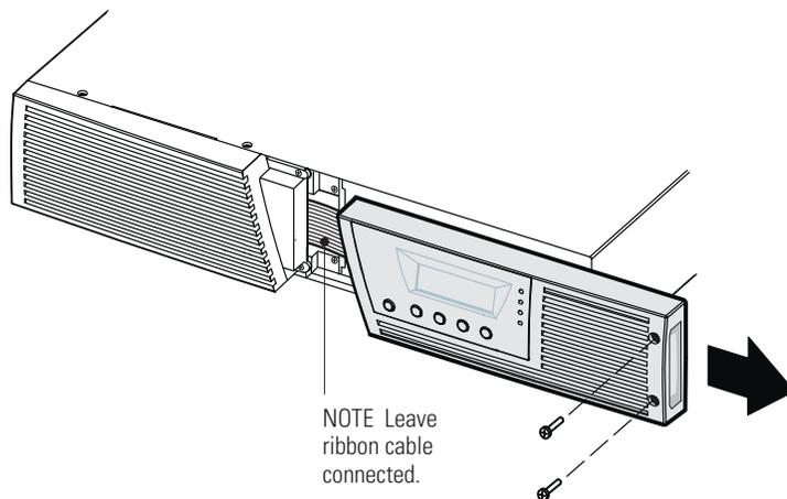
**Figure 23. Removing the UPS Right Front Cover**
