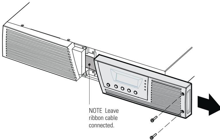
**Figure 9. Removing the UPS Right Front Cover**
