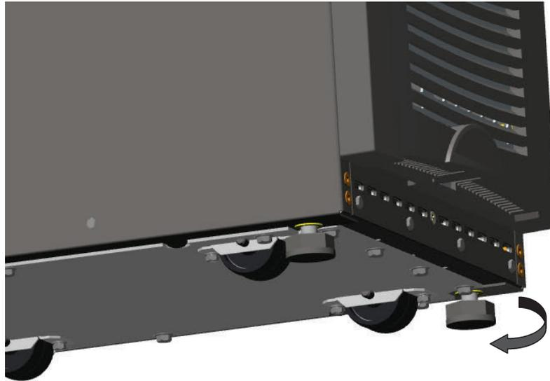
2. Attach the stabilizing bracket to the bottom of the cabinet rear panel using the retained hardware from the shipping pallet according to the cabinet configuration:
