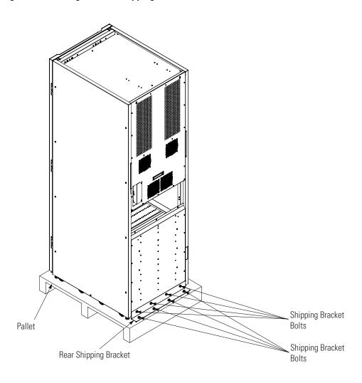
Figure 9. Removing the Rear Shipping Bracket
