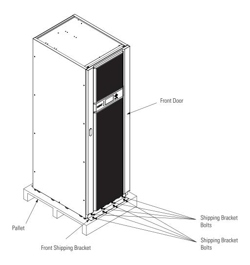
Figure 7. Removing the Front Shipping Bracket
