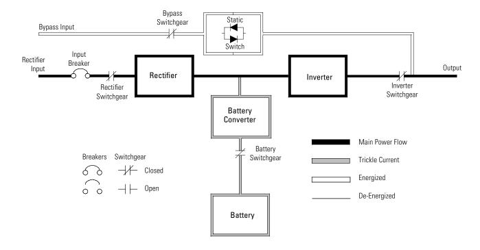
If the UPS becomes overloaded or unavailable, the UPS switches to Bypass mode. The UPS automatically returns to Normal mode when the overload condition is cleared and system operation is restored within specified limits.
