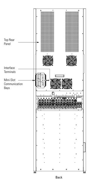
Figure 17. Interface Terminal Detail (Terminal Cover Removed)
