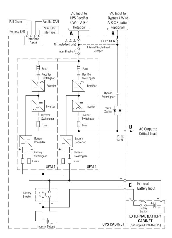
Figure 37. UPS System Oneline – Internal and External Batteries
