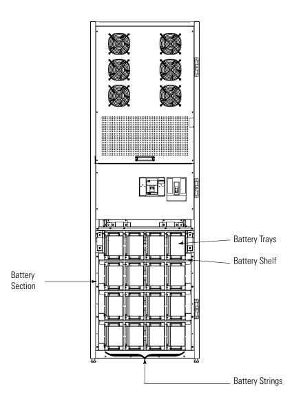
**NOTE** The Eaton 93E-40 model has battery strings installed on three shelves. The Eaton 93E-60/40 and Eaton 93E-60/60 models have battery strings installed on four shelves.
