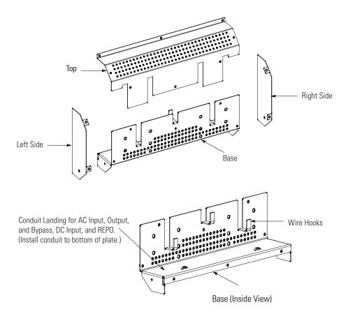
**NOTE** Do not install the Power Terminal Cover Left and/or Right Side covers if wiring adjacent ancillary cabinets (such as an EBC or IAC) using the power terminal base wiring channel.
