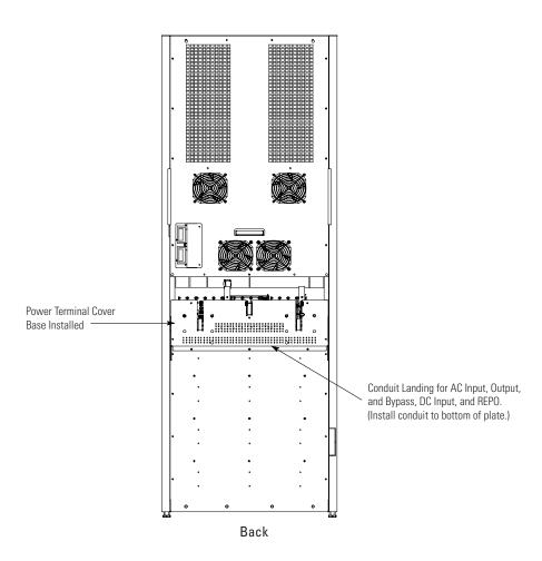
Figure 12. UPS Power Terminal Cover Base Installation and Conduit Landing Wire Entry Locations
