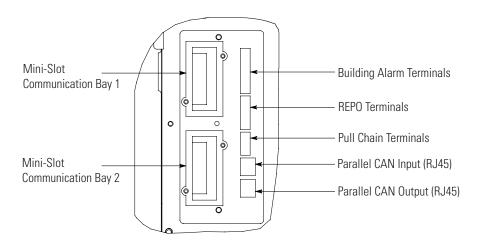
Figure 18. Building Alarm Terminal Block Connector Assignments
