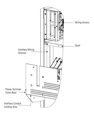
Figure 20. Interface Conduit Landing and Wiring Channel
