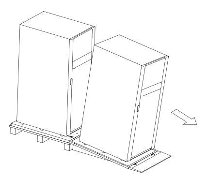
Figure 10. Rolling the Cabinet Down the Ramp
