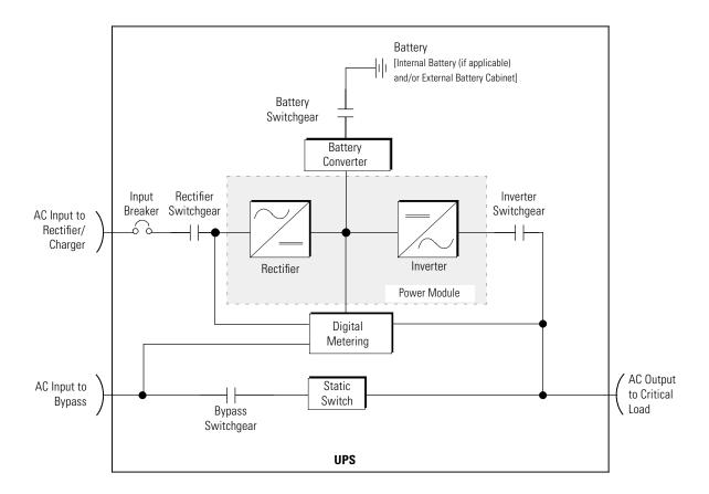
The emergency bypass consists of a continuous static switch, and a bypass switchgear. The bypass switchgear is located in series with the static switch. The static switch is armed and ready during normal operation.
