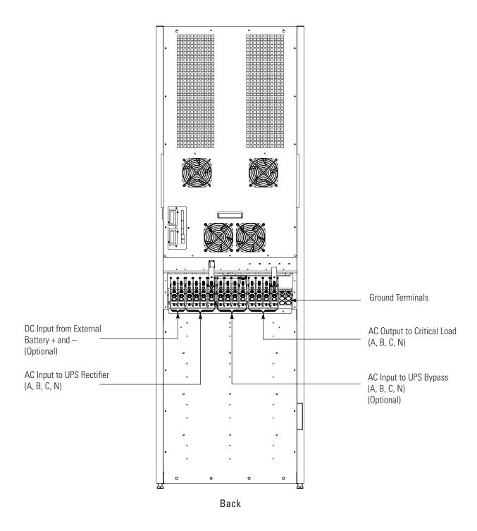
Figure 14. Power Terminal Detail
