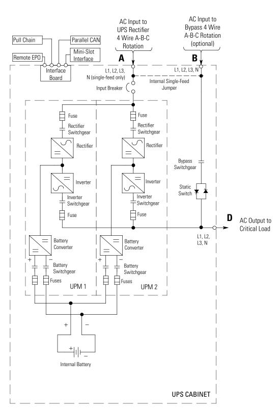
Figure 35. UPS System Oneline - 93E-40 Internal Battery (No External Battery Capability)
