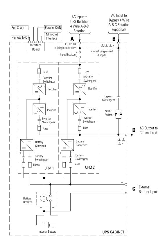
Figure 36. UPS System Oneline – Internal Battery and External Battery Capable
