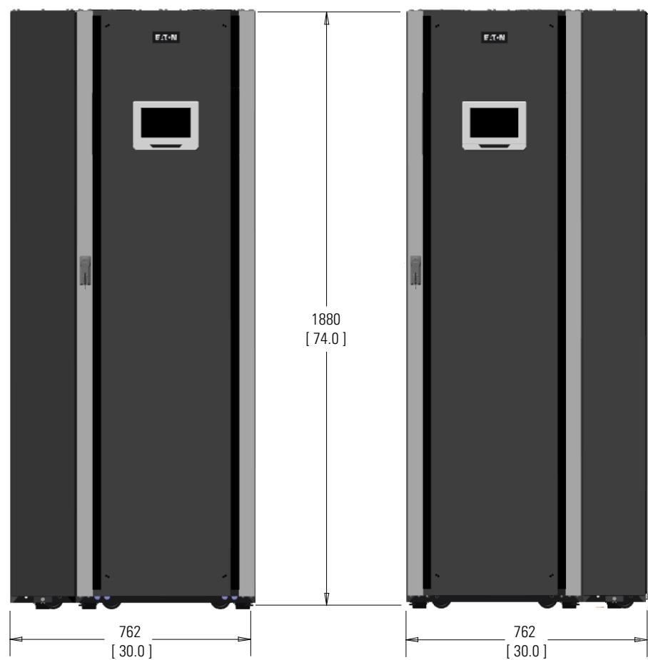
Front UPS With Left-Mounted Sidecar
