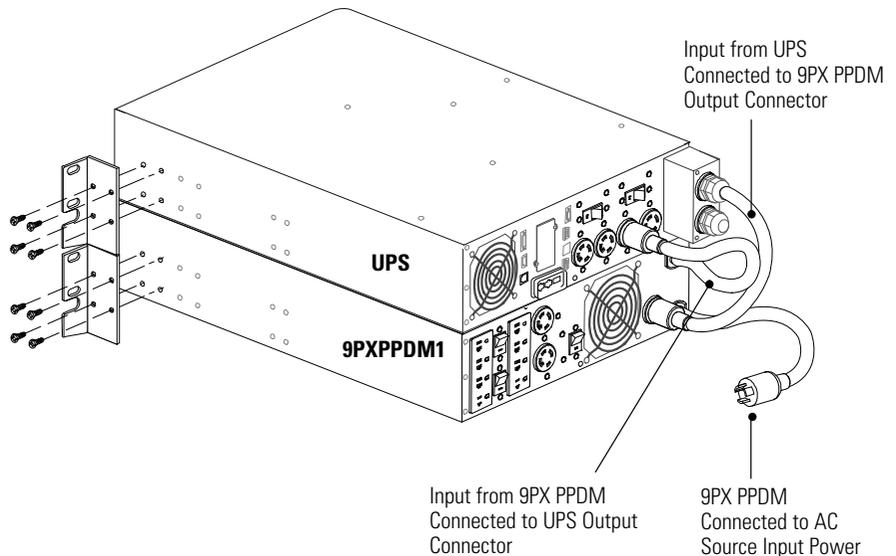
**Figure 30. 9PXPPDM1 with 9PX5000 or 9PX6000 UPS (Kits 9PX5KP1 and 9PX6KP1)**
