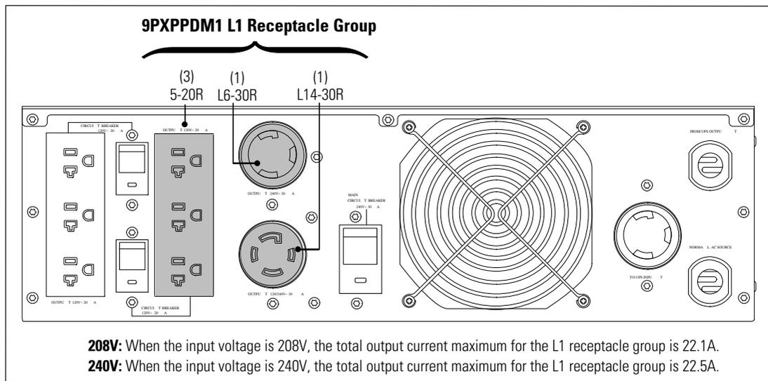
Figure 27. 9PXPPDM1 L1 Load Output Limits
