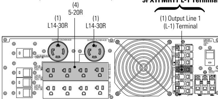
**208V:** When the input voltage is 208V, the total output current maximum is 41.7A for either the L1 receptacle group or the L-1 terminal.
