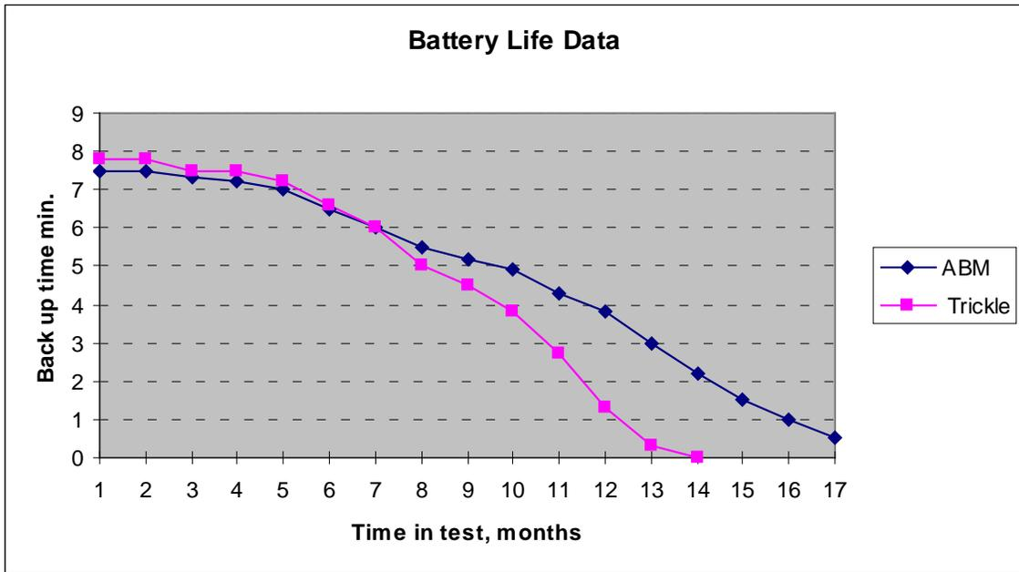
**Figure 2:** Accelerated Life Testing of ABM at 40 degrees C
