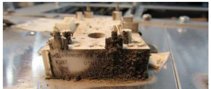
Close-up photo of an IGBT inside a power module that overheated due to effects of dirt and dust collection over time.
