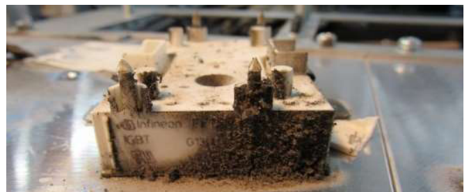
Close-up photo of an IGBT inside a power module which overheated due to effects of dirt and dust collection overtime.
