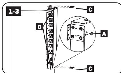
**1-4 Under-Counter Mounting:** Use 4 screws **A** to attach each of the 2 mounting brackets **B** to the PDU as shown. Mount the PDU under the counter by inserting 2 or more user-supplied screws **C** through the mounting brackets **B** and into secure mounting points.
