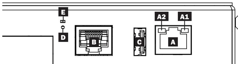
**A Ethernet Port:** RJ45 jack connects the PDU's Network Interface to the network using a standard Ethernet patch cable. LEDs **A1** and **A2** indicate the operating conditions (shown in the table below).
