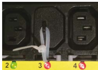
Cap secures in place with cable tie
