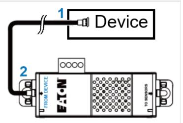
**STEP 1** – Connect the Ethernet cable to the RJ45 port of the Device.
