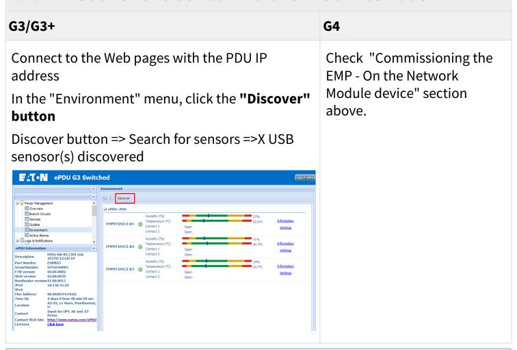
The Environment menu appears only when an EMP is connected to the Rack PDU
