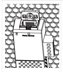
To mount the EMP on the rack, use the supplied screw, washer and nut. Then, mount the EMP on the screw and tighten it.
