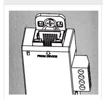
To mount the EMP on the wall close to the rack, use the supplied screw and screw anchor. Then, mount the EMP on the screw and tighten it.
