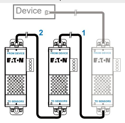
**STEP 1** – Connect the Ethernet cable to the "TO SENSORS" port of the first EMP, and to the "FROM DEVICE" port of the second EMP.
