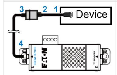
**STEP 1** – Connect the "USB to RS485 converter cable" to the USB port of the Device.
