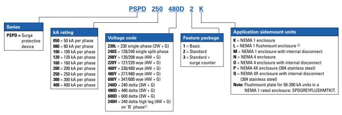
Example: PSPD250480D2K = PSPD Series, 250 kA per phase, 480D voltage, standard feature package, housed in NEMA 1 enclosure a Please consult the factory for 240 delta high leg (4W + G) applications with high leg on 'C' phase. b NEMA 1 flushmount units are available in 50-200 kA ratings only.
