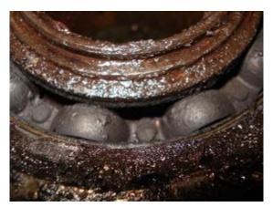
Figure 1: Incompatible Grease Failure
