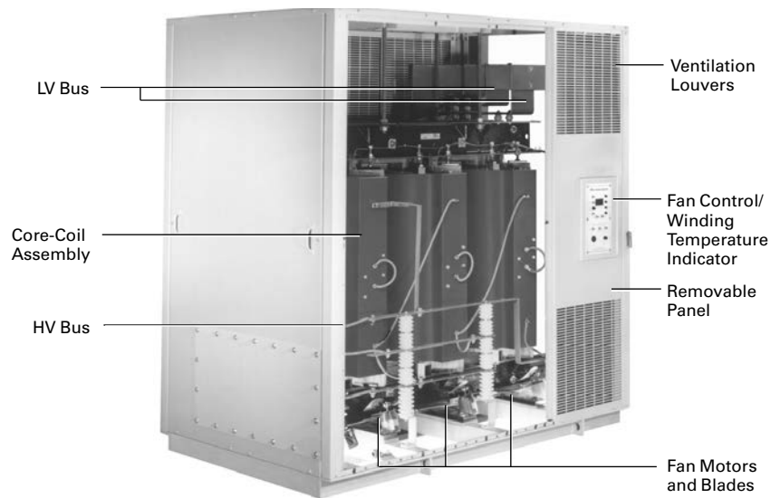
Cast Coil Substation Transformer
