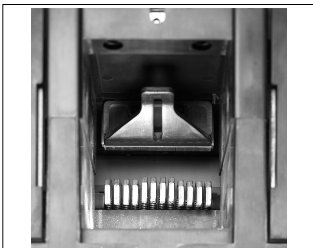
Figure 6-3: Primary Contacts with Circuit Breaker Open (Not Used for Contact Wear Inspection)
