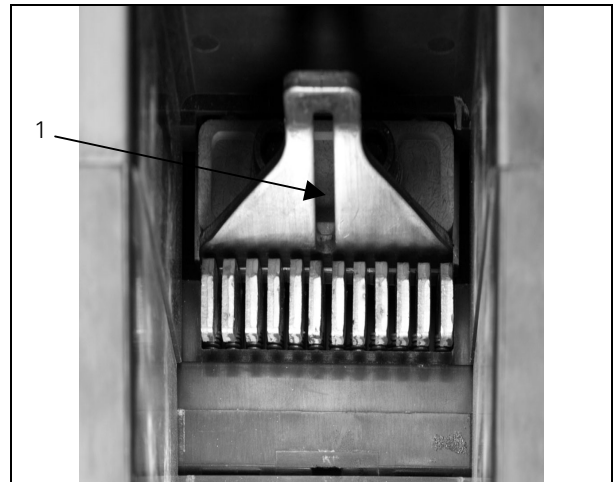
Figure 3-14: Integral Arc Runner Viewed From Top of Arc Chamber (Arc Chute Removed, Circuit Breaker Closed)
