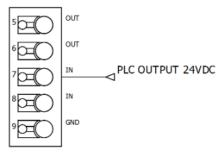
To switch the PXS24 remotely, one of the PXS24 inputs (pin 7 or 8) can be connected directly to a controller output. With this type of connection the PXS24 can also be used as a protective relay.
