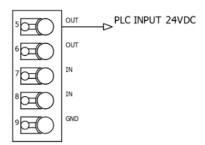
To monitor the status of the PXS24 remotely, one of the PXS24 outputs (pin 5 or 6) can be connected directly to the input of a variety of controllers.
