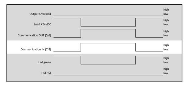
The path highlighted in white can be controlled by the user; the paths highlighted in gray will change in line with the changes to the white path.
