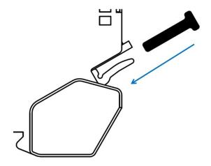
The PXS24-BB... busbar is designed for currents up to 80 A.
