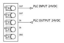
The PXS24 can be fully monitored via a controller if one of its inputs (pin 7 or 8) is connected to a controller output and one of its outputs (pin 5 or 6) is connected to a controller input. With this type of connection the PXS24 can also be used as a protective relay.
