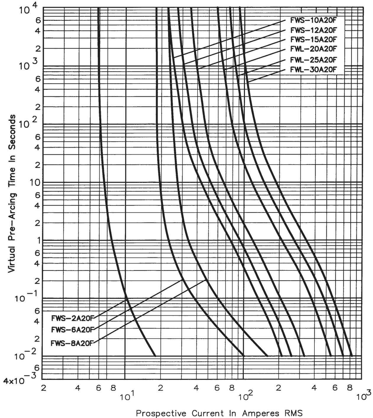
**Minimum Melting** Time-Current Characteristic Curves
