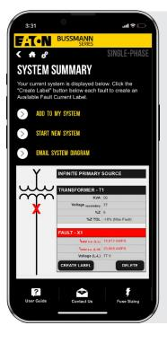
Eaton's Bussmann<sup>®</sup> series FC<sup>2</sup> Available Fault Current Calculator is a simple-touse mobile and web-based application that calculates single- and three-phase system available fault current.
