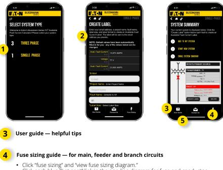
Click each blue "hot spot" link in the one-line diagram for fuse and conductor sizing diagram
