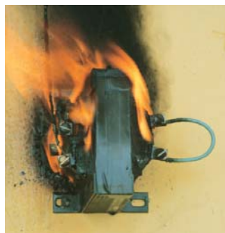
This photograph vividly illustrates the effects of overcurrents on electrical components when protective devices are not sized to the amp rating of the component.
