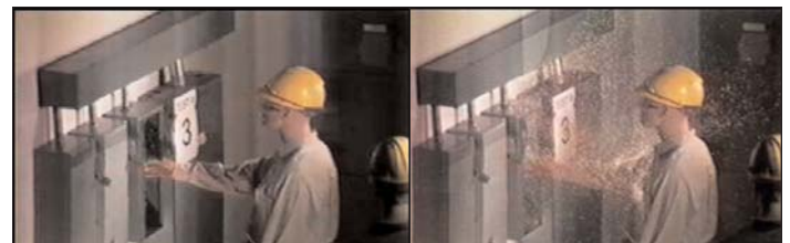
Test 3 – Same test circuit as the prior photos, to the left, except the circuit is protected by KRP-C-601SP Cooper Bussmann Low-Peak® Current-Limiting Fuses. In this case these fuses limited the current and the fuses cleared in less than a \frac{1}{2} cycle.
