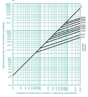
Low-Peak Class J, Dual-Element Time-Delay Fuses LPJ\_SP
