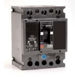
combination controller. MCPs are short-circuit tested only in combination with a motor controller and overload device. They are not labeled with an interrupting rating by themselves. Per NEC® 430.109 exception 7, they may be used as a motor disconnecting means when part of a listed combination motor controller.
