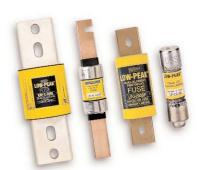
from 10,000 amps to 300,000 amps. These fuses are listed for branch, feeder, and main protection. In a motor circuit they provide branch circuit, short-circuit, and ground fault protection. In addition, enhanced overcurrent protection such as back-up overload and Type 2 "No Damage" protection can be provided with the selection of certain fuse sizes and types.
