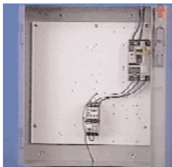
Photo 1 Before Test: MCP as motor branch circuit protection for 10HP, IEC Starter with 22,000 amps available at 480V.
