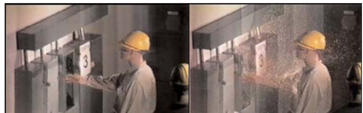
Test 3 – Same test circuit as the prior photos, to the left, except the circuit is protected by KRP-C-601SP Cooper Bussmann Low-Peak® Current-Limiting Fuses. In this case these fuses limited the current and the fuses cleared in less than a \frac{1}{2} cycle.
