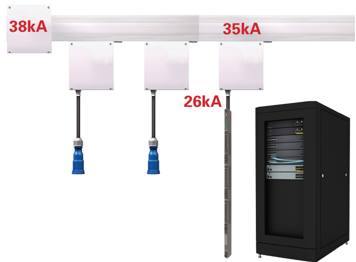
Figure 1: Typical data center busway, busway drop units and rack PDU with high fault current levels.
