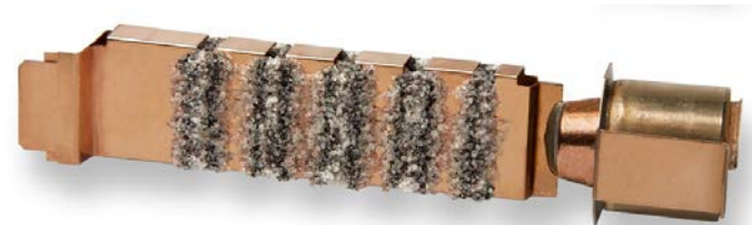
Figure 3.1.3.2.e Arc-quenching filler material helps suppress the arcing by melting and forming folgurite.
