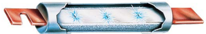
Figure 3.1.3.1.d When subjected to a fault current, several sections of the fuse link melt almost instantly.
