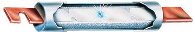
Figure 3.1.3.1.b Under sustained overload, a section of the link melts and an arc is established.
