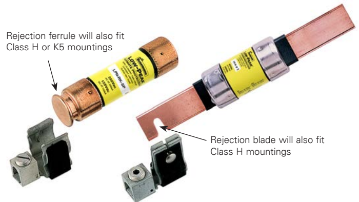
Figure 3.1.6.1.c Class R fuse rejection clips (restriction on the ferrule or notch on the blade) that will only accept Class R fuses.
